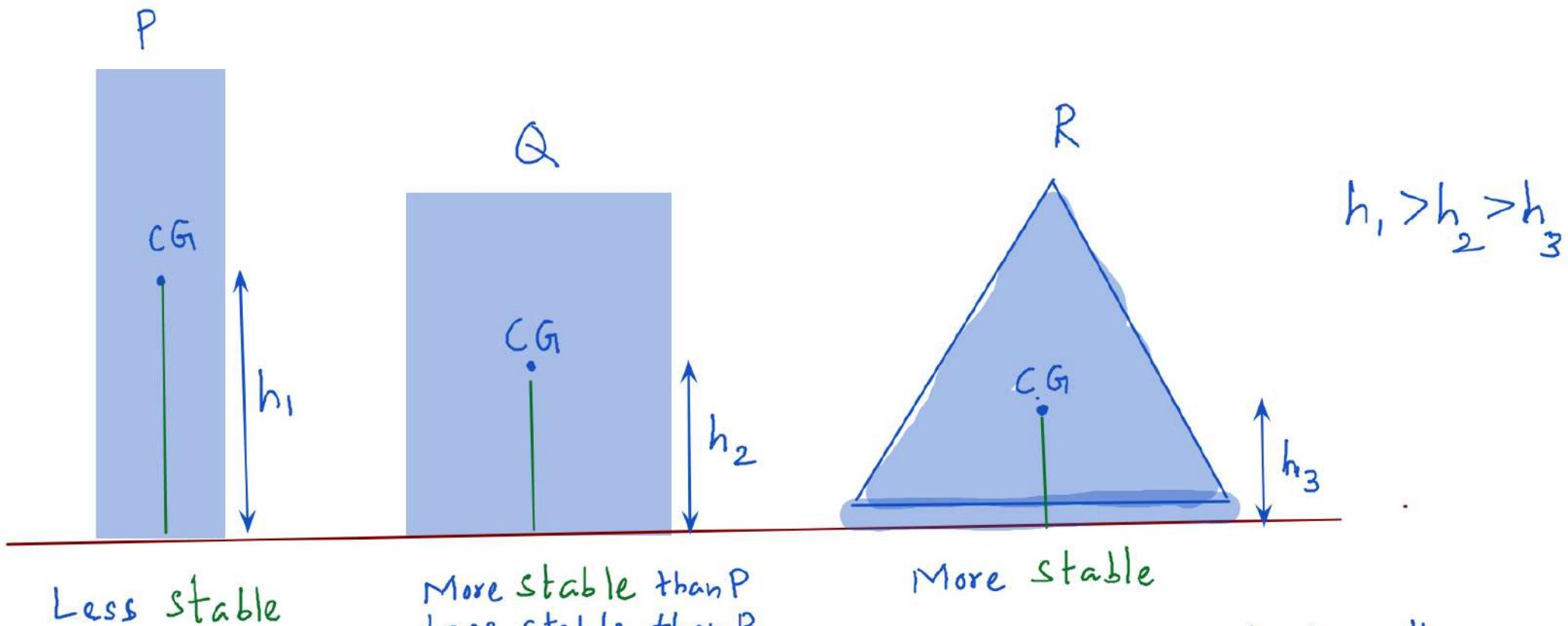
In case of a stable object, greater the height of centre of gravity from the ground, lesser is the stability of the object and vice-versa.
