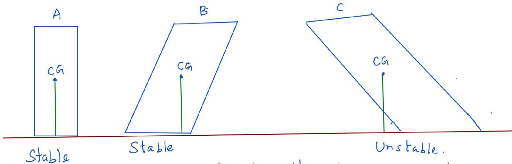
The line passing through centre of gravity and perpendicular to the ground touch the bottom of the object for a stable object, does not touch the bottom of the object for an unstable object.
