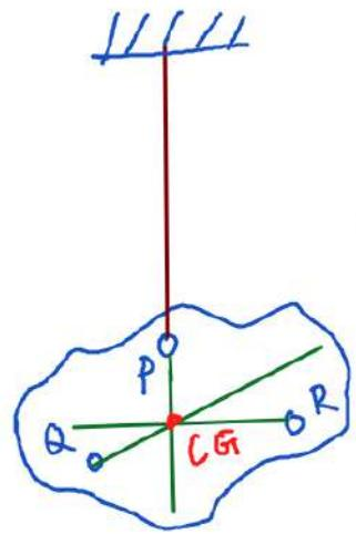
Make three holes at three different sides of the lamina and suspend it through one of the hole, draw the line extending the irregular direction of suspended thread. lamina Repeat the experiment with other two holes. All the lines meet at one point called centre of gravity of the irregular lamina.
