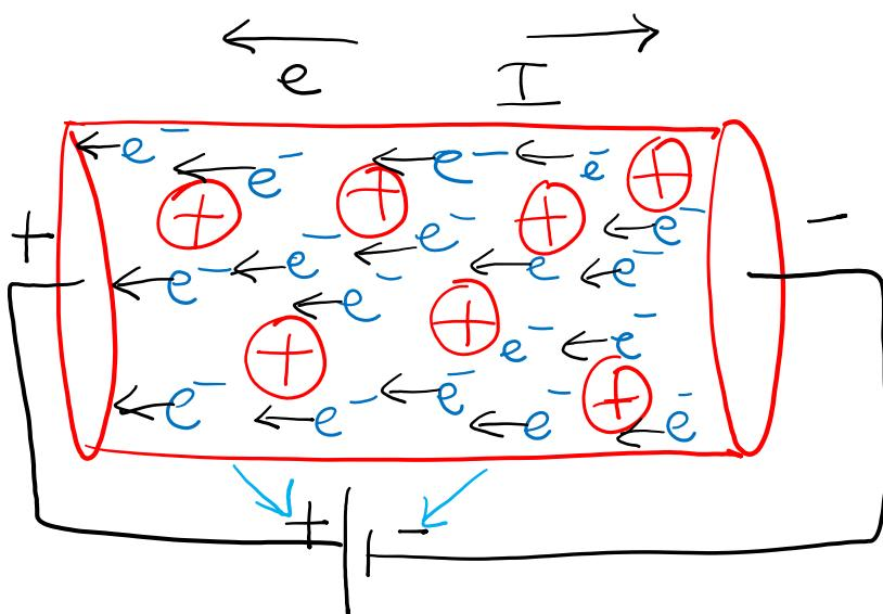
electrons drift because applied voltage as it collides repeatedly with heavy + atoms.
